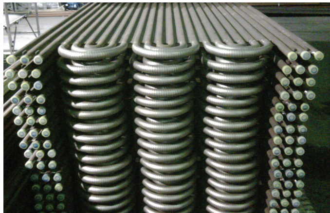
Nappes serpentins de surchauffeur
