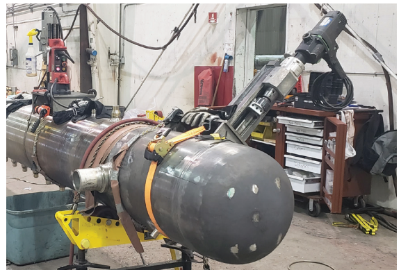
Drilling gamma ports and weldolets
