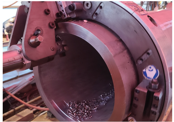
Counterbores using clamshell lathes
