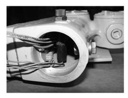
6. Remove the red LED indicator assembly from the housing.
