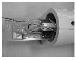
10. Remove the wire connector by sliding the connector out of the circuit board.
