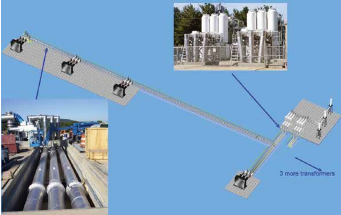
Bethlehem Power Plant, Pennsylvania, USA 550kV, 2000A Complete Substation From Transformers to Transmission Lines
