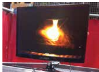
Nozzlefuse 624: The built-in camera provides real-time visual control of the overlay
