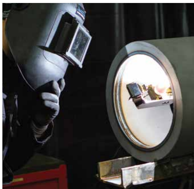
WSI offers a unique, fully automated repair solution for the Nozzle ID covering a range from 2 to 24 inches
