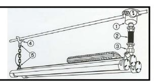
Flexible mounting provides free swing and impact protection.
